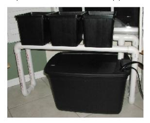
**16.** Now to make the "spaghetti" feeder lines. The large 1/2" tubing that comes up from the pump in the reservoir: arrange it so that it runs at the back top edge of the 3 buckets, and tape in place temporarily.
