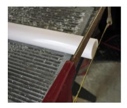
**2. Next, a word about PVC cement.** You will apply a nice coat of glue to each PVC piece before pushing them together. *Once you attach them together, you have all of* **5** *seconds to get it seated properly before a permanent and unbreakable bond is set.* If you screw it up, throw in the trash and start over. (Hence the advice to buy a couple extra elbows and t-piece).
