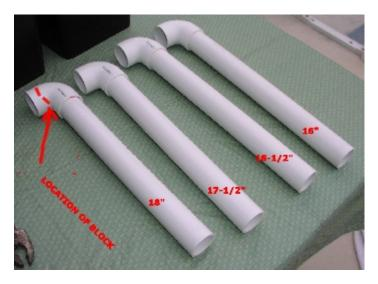
**6.** Now glue the two longer legs to the back (drain) rail (the assembly with the T pc glued in). The 18" pc (with the block glued in the elbow) goes on the plain end of the rail. The 17 1/2" leg goes on the T-pc end of the rail. First you will do a dry run. The legs need to be flat (& parallel), but the t-piece will angle in, to drain into the reservoir. This is what you are attempting to do:
