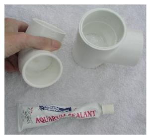
**4.** Okay, time to glue up the back rail. For this, use the 31" & 2" pieces of straight pipe, and the "T" piece with the "block" glued in one side. Do not put the elbows on at this time. Make sure you put the T-piece on with the "block side" towards the outside, the 2" piece. This is how it should be assembled:
