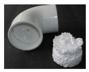
**3.** Next, push one styro block into one elbow piece and do the same for one end of the "T" piece. Push in far enough so you leave enough room for the straight pipe to fit in there later. Apply a thick coat of silicone sealant on top of the block, and around the sides of it. Allow it to set up, then apply a second coat. The idea is, you want it totally blocked off so no moisture can get through. *Tip: do not use PVC cement for this. It melts the styrofoam. Trust me.*
