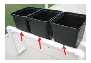
**11.** Using the 7/8" spade bit or a 1" hole saw bit, drill the three holes in the very top of the PVC pipe. This is where the Bato bucket drain elbows will fit into the drain pipe.
