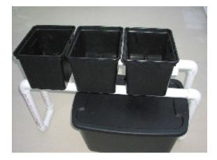
**13.** The remaining 6" piece of PVC pipe is the drain pipe extension. Glue it into the down port of the T-piece. Then using the 2-¼" hole saw, cut a hole in the reservoir lid right where the drain port extension hits the lid, so it will enter it. Cut a smaller 1" hole in the front corner as shown. This is where the hose is going to come up from the pump to the feeder lines.
