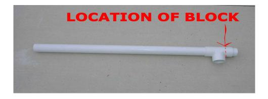
**How to use PVC glue:** apply to both pieces, then push them together, all the way in. Hold jammed all the way together for about 5 seconds to set the glue. It is now permanently bonded.
