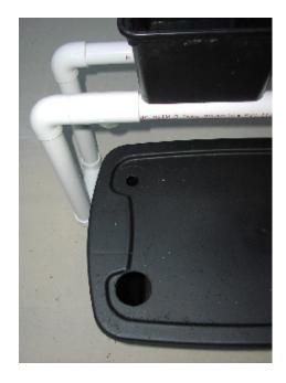
**14.** Push one end of the 6 foot  $\frac{1}{2}$  inch irrigation tubing onto the outlet port of the pond pump. If it fits too loose, you must secure it with a zip tie so it doesn't come off during assembly and operation. First push the pump electrical plug up through the bottom of the reservoir lid, then the  $\frac{1}{2}$ " irrigation tubing through the same hole. See photos below.
