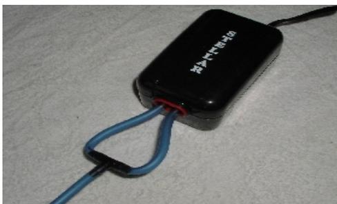
This air pump has two outlet ports. If yours does too, then buy the "T" adapter and tie in both ports to one airstone. No use wasting half those precious bubbles!
