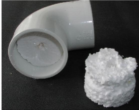
**3.** Next, push one styro block into one elbow piece and do the same for one end of the "T" piece. Push in far enough so you leave enough room for the straight pipe to fit in there later. Apply a thick coat of silicone sealant on top of the block, and around the sides of it. Allow it to set up, then apply a second coat. The idea is, you want it totally blocked off so no moisture can get through. *Tip: do not use PVC cement for this. It melts the styrofoam. Trust me.*
