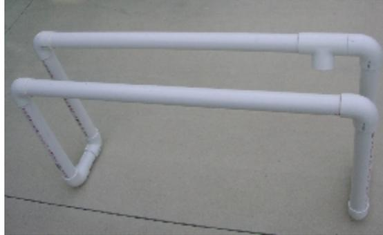
**10.** Now it's time to drill the drain holes in the back drainage rail (the one with the t-piece). Set the three Bato buckets onto the frame so they line up evenly between the elbow and the T-piece and mark on the PVC pipe where the drain holes come out:
