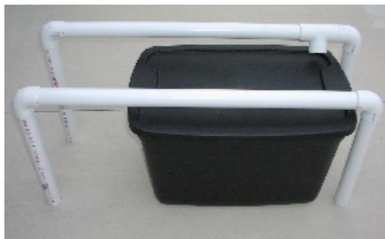
**9.** Next add the two 5" pieces to the bottoms of the legs. Glue one elbow on each end of each of the 5" cut pieces, making sure to seat them all the way in for each joint. Then glue to the bottom end of the two assembled frames. The two taller legs (18" and 16-1/2") go to one "U" and the two shorter legs (17 1/2 and 16") go to the other "U". This is what it looks like all glued up:
