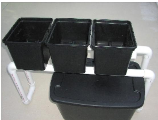
**13.** The remaining 6" piece of PVC pipe is the drain pipe extension. Glue it into the down port of the T-piece. Then using the 2-1/4" hole saw, cut a hole in the reservoir lid right where the drain port extension hits the lid, so it will enter it. Cut a smaller 1" hole in the front corner as shown. This is where the hose is going to come up from the pump to the feeder lines.
