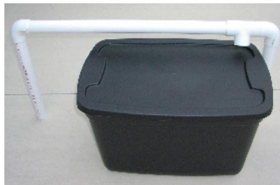
**7.** First assemble as a dry run, making sure the legs lie flat, with the top pc angled in slightly. Use a marker to show where the pieces line up before gluing them home. Push flat on the floor as you glue it together so it is perfectly FLAT.
