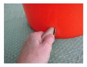
**2.** Insert the grommet into the hole. Work carefully and seat it so it flares out on the inside and the outside of the bucket. It will fit a little loose at this point. The insertion of the elbow piece later will tighten up the seal.
