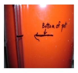
**9.** Set the bucket up off the floor on a sturdy table or other support; (its final resting place). You need to have it elevated so you can drain solution from it easily. Start adding water one gallon at a time. Check for leaks at the elbow. Stop after adding each measured gallon and mark that on the clear level indicator tube, so you will have the volume indicated once the bucket is set up.
